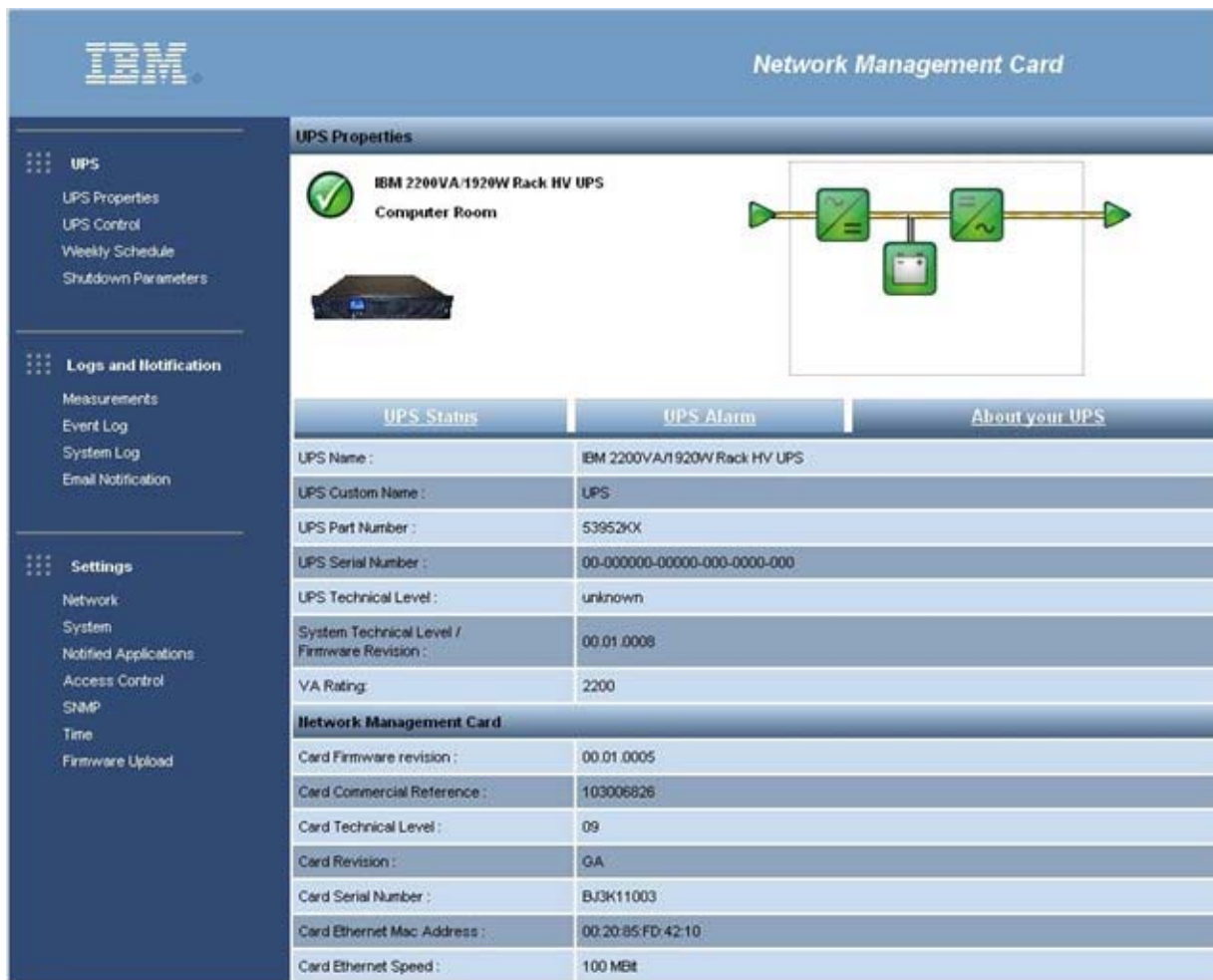
Figure 8. IBM LCD UPS Network Management Card (NMC) UPS properties window
